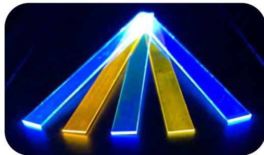
LUMINESCENT CONCENTRATORS USED AS EFFICIENT PUMP SYSTEMS FOR LASERS AND MASERS, AND TO ENHANCE LED BRIGHTNESS IN PHOTONIC APPLICATIONS (NORTHUMBRIA UNIVERSITY).
