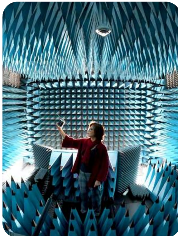
BRADFORD-RENDUCHINTALA CENTRE: ANECHOIC CHAMBER
